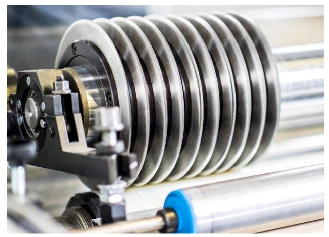
The new slitting and winding machine from ROBUST HABICHT & HEUSER is a perfect solution for the longitudinal cutting off the roll.
